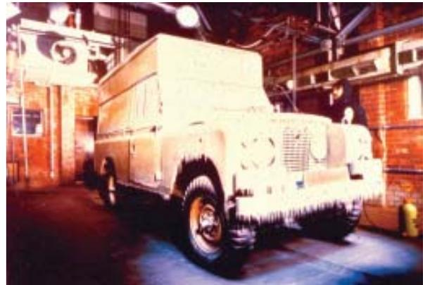
Figure 1-9 Climatic test on MIL vehicle
