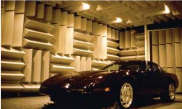
Figure 1-29 Noise test in hemi anechoic room
