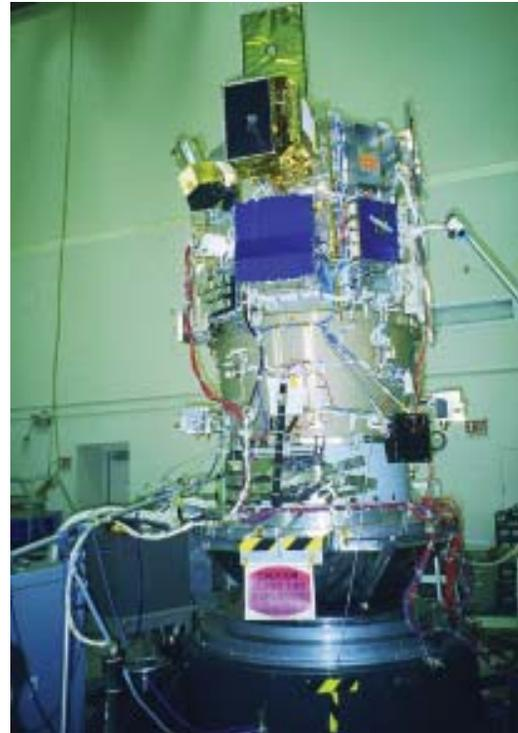
**Figure 1-11 Vibration test on satellite**
